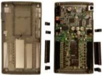
Step # 3: To remove PCB from enclosure use small flat head screw driver to depress the plastic tabs holding PCB in place allowing PCB to be easily separated from plastic.
