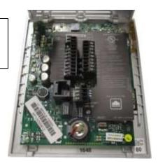
Step # 3: Remove screws holding PCB to plastic housing.
