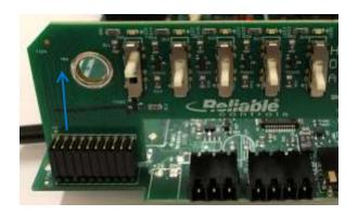
Step # 7: Slide the circuit board away from and out from the aluminum enclosure to discard.
