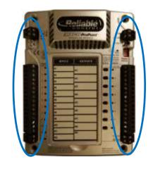
Step # 2: Using small flat head screw driver depress the two plastic tabs on side of controller and pull two sides apart gently.
