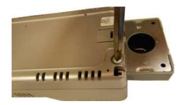
Step # 3: Depress plastic tab to release motor using flathead screwdriver (if applicable)
