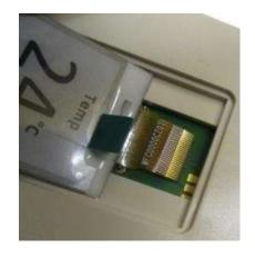
Step # 4: Detach flex strip that was underneath LCD from plastic housing.
