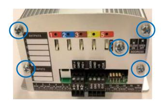
Step # 3: Turn the unit to the other flat side and with a Phillips head driver, Remove 2 Phillips head screws
