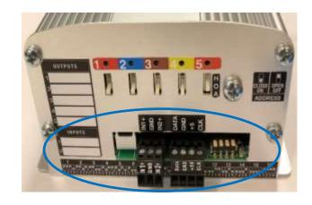
Step # 2: With a Phillips head driver, Remove all 5 Phillips head screws
