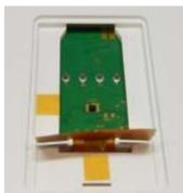
Step # 4: Flex or bend the plastic enclosure in order to release the PCB from the four clips shown.
