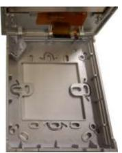
Step # 7: Remove LCD by inserting small flathead screwdriver between LCD and plastic and prying apart gently.
