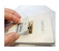
Step # 3: Disconnect flex strip by pulling black tab on connector to release flex strip.
