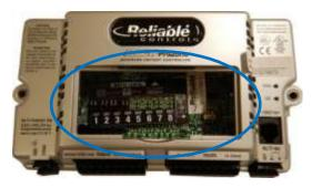
Step # 3: Remove PCB by pulling on plastic tab of enclosure and pushing gently from other side (through top plate opening).
