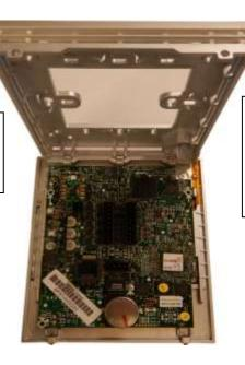
Step # 4: Lift PCB from bottom and disconnect ribbon cables from connectors.
