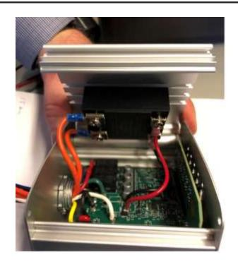
Step # 5: With a Phillips head driver, loosen the two screws on the top of the aluminum enclosure to slide the relay away and off the top. Remove any remaining fasteners.
