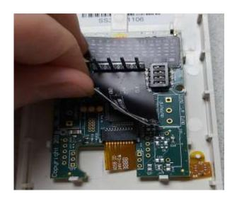
Step # 4: With a Phillips screwdriver, remove two screws from printed circuit board (on applicable options)
