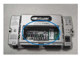
Step # 3: With a small screwdriver, place the slot between the plastic housing and circuit board and push out until the tab releases the circuit board.
