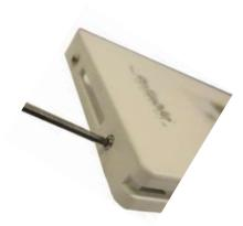
Step # 2: Remove glass by inserting small flathead screwdriver between plastic and glass and gently prying apart to lift up.
