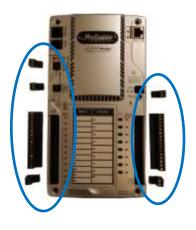
Step # 2: Using small flat head screw driver depress the two plastic tabs on side of controller and pull two sides apart gently.
